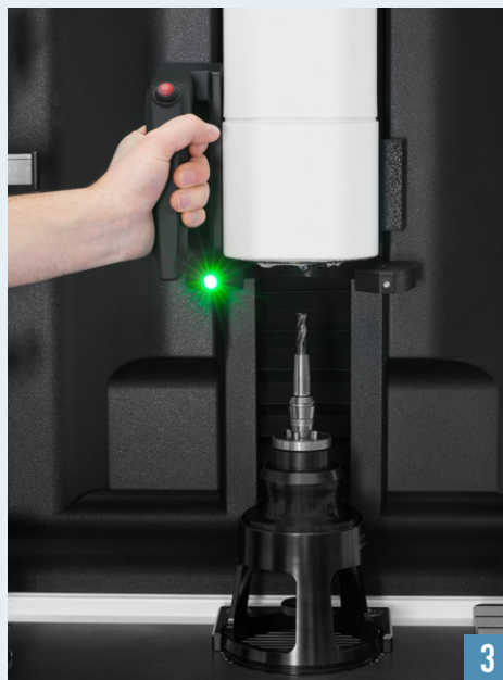
Cooling of shrink fit collet with temperature control
