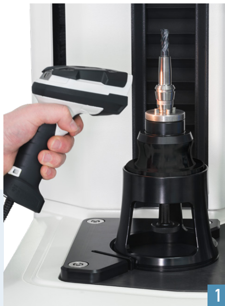
Length presetting and scan of Data-Matrix Code for automatic identification of shrinking parameters
