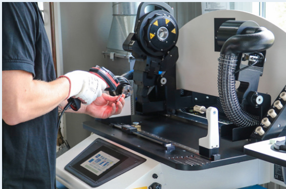
The operator reads the QR code on the shrink fit collet with a hand scanner. The shrink fit machine is then provided with all important parameters.
