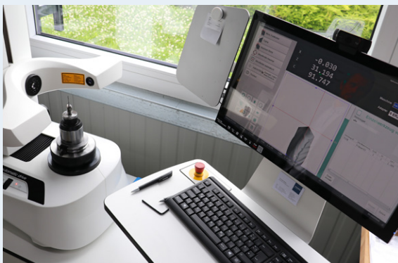
The HAIMER Microset UNO 20|40 automatic drive tool presetter features an image editing system and automatic tool measurement in three axes.
