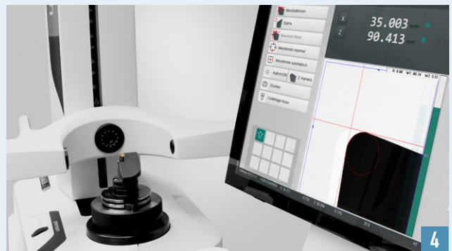
Common adapters like VDI, Trifix, PSC, HSK with 4 x 90° indexing
