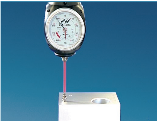
Measure surface flatness
