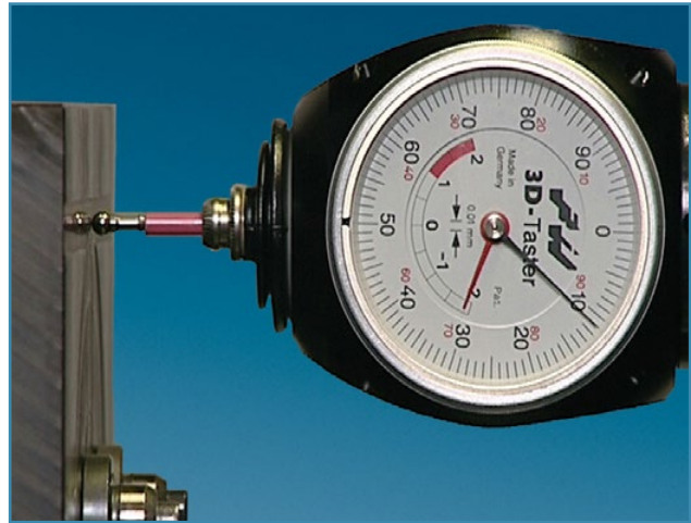
Tram in your work piece or fixture to your machine
