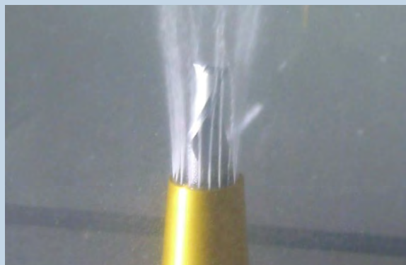
Slip-on sleeve with nozzles – ineffective cooling, coolant does not reach the cutting edges
