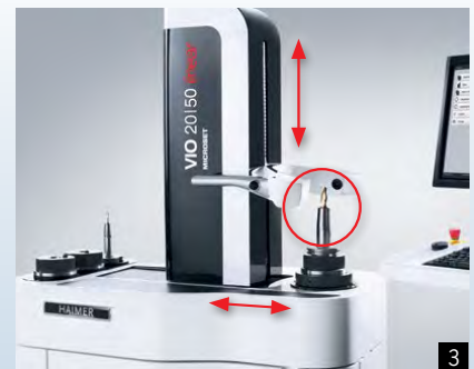
1: Second camera for measuring the center of rotation (optional) 2–3: Fully automatic axis drive via modern linear technology
