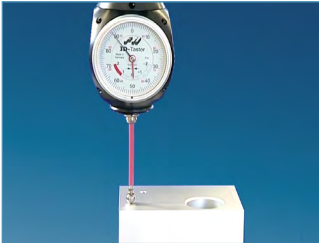
Measure surface flatness
