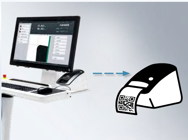
After measuring the tool, a label with the QR code is printed
