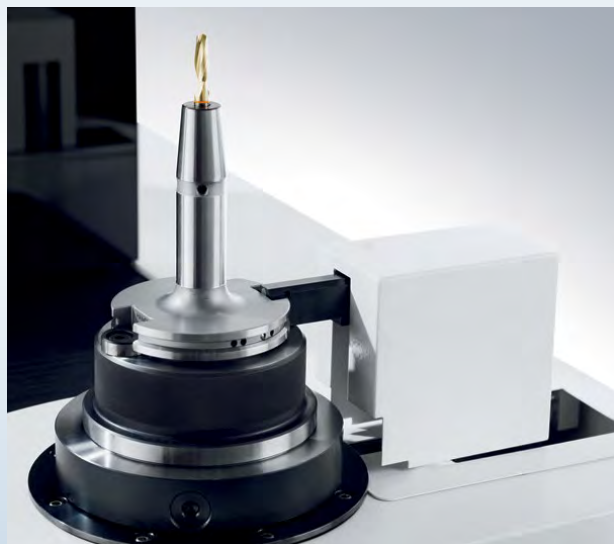
Automatic positioning of the read/write head
