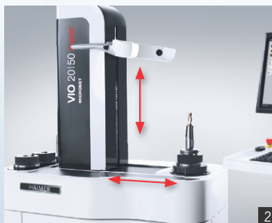
1: 第二摄像头用于测量车刀的中心高度(选配)/Second camera for measuring the centre of rotation (optional) 2 + 3: 先进的线性电机技术协助全自动的驱动各轴/Fully automatic axis drive through modern linear technology
