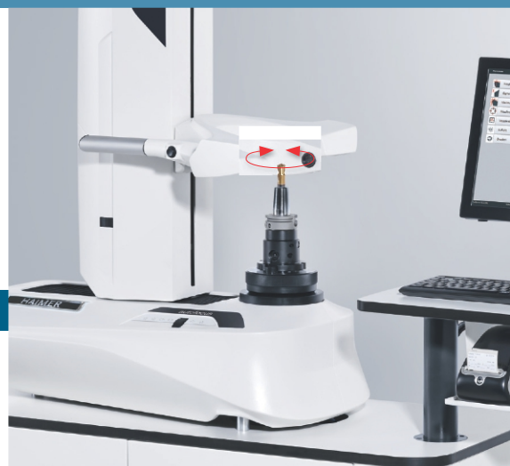
自动聚焦切削刃 Automatic cutting edge focusing
