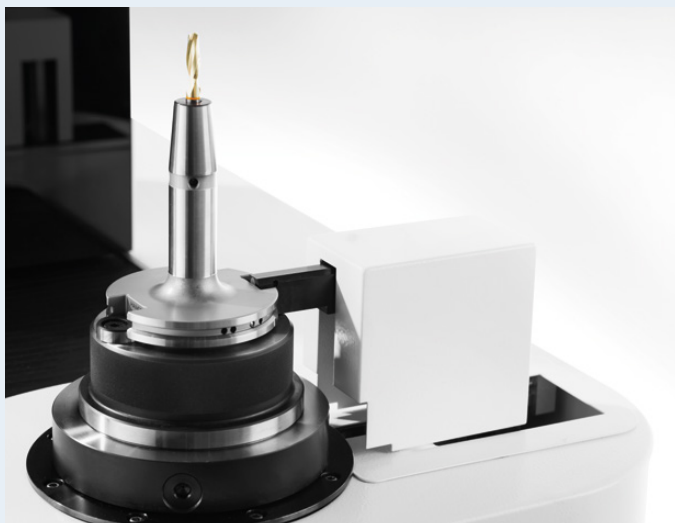
Automatic positioning of the read/write head
