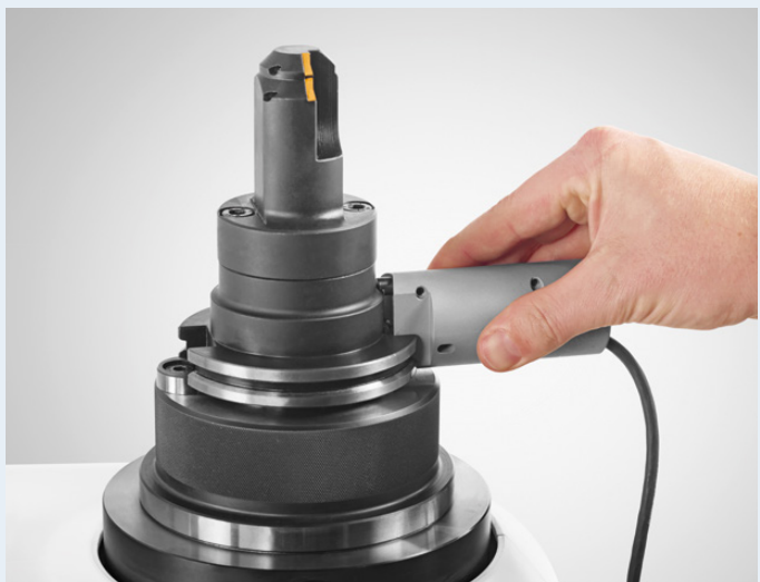
Manual positioning of the read/write head
