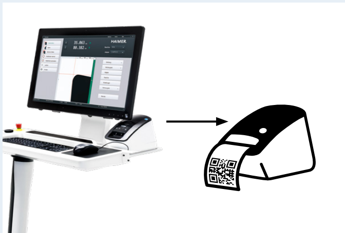
After measuring the tool, a label with the QR code is printed.
