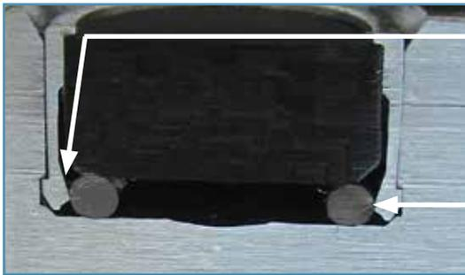
Sleeve is clamped by form and press fit into the tool holder
