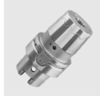
**Finally there is a holder for heavy machining that can replace the Weldon tool holder. The Heavy Duty Chuck is a shrink fit chuck designed for extreme cases. The contour is optimized for highest rigidity and clamping force.**
