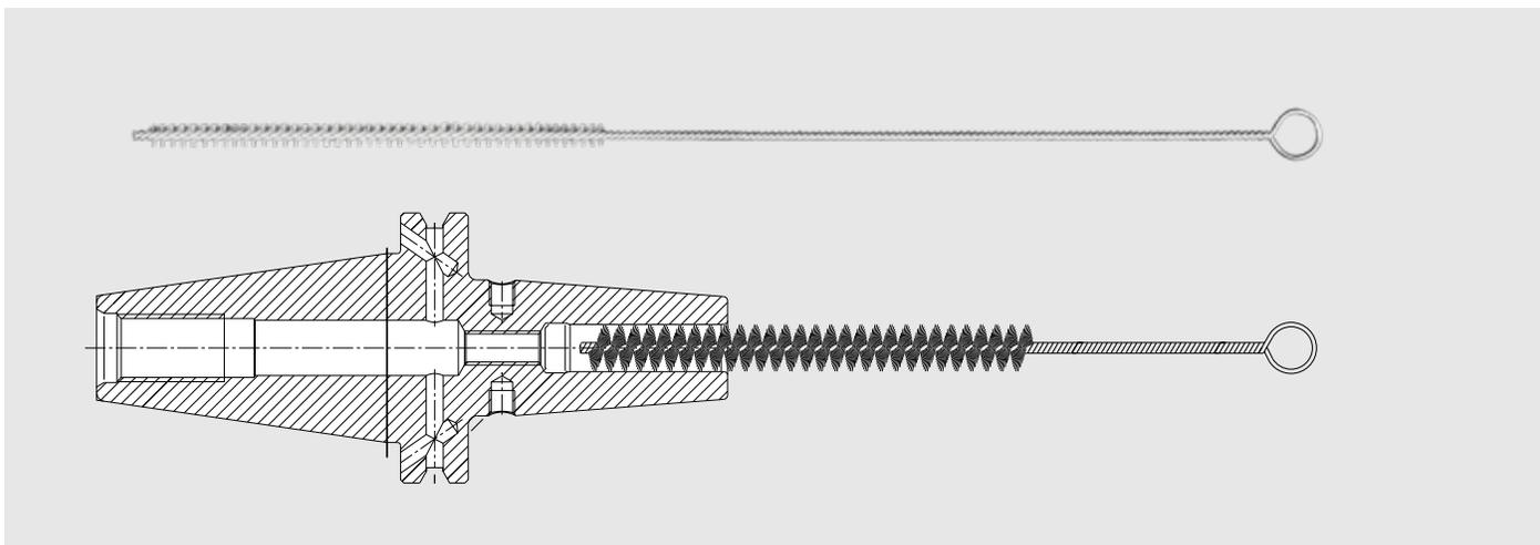
In order to achieve the best possible shrink fit connection, a grease free socket and shank is necessary. The cleaning can be done by a cold solvent (e.g. brake cleaner). An appropriate cleaning brush is necessary to clean the socket of the Shrink Fit Chuck.
