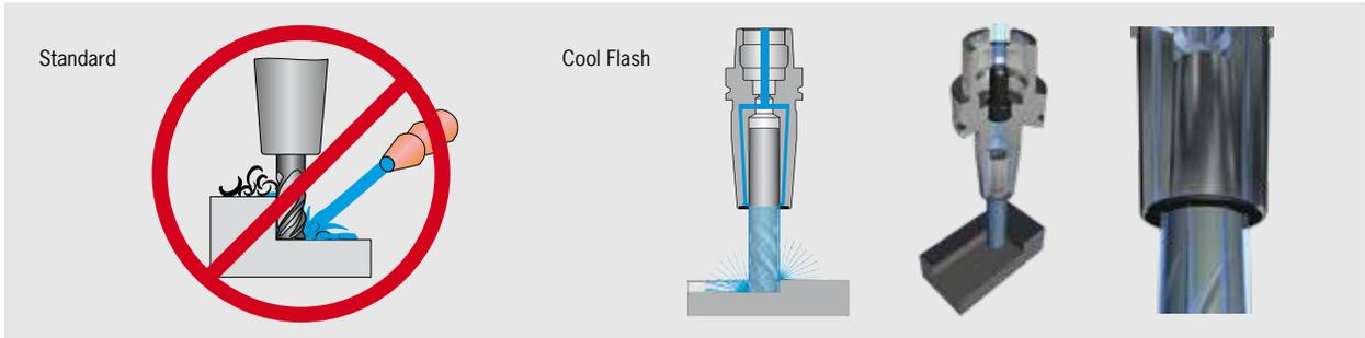
True to the slogan “make good things even better”, HAIMER has developed the Cool Flash system out of the existing Cool Jet system. The Cool Flash design directs coolant into T-slots at the nose of the holder and works with the centrifugal force of the rotating tool to lead the coolant along the shank of the cutter and directly to the flutes at any speed.
