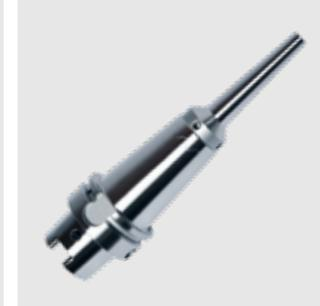
The Power Mini Shrink Chuck is perfect for 5-axis machining in the die & mold and in the medical industry. Very slim at the top like the HAIMER Mini Shrink Chucks, the Power Mini Shrink is reinforced at the base. This allows for efficient milling with an angled tool, even at long protruding lengths.
