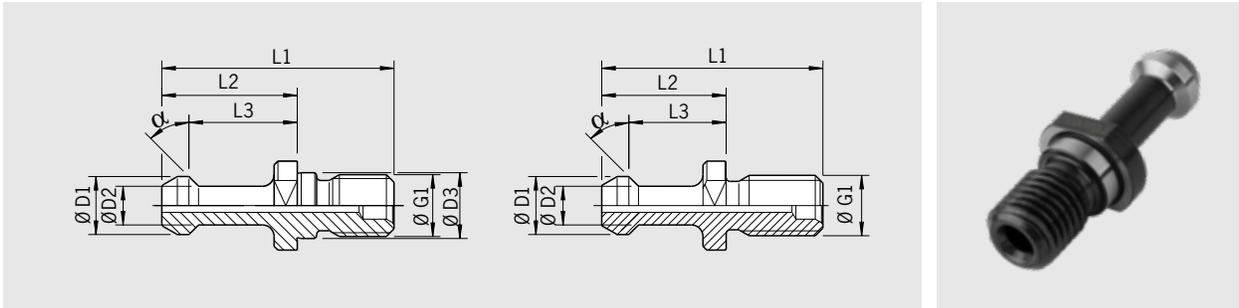
Version with ground pilot is used to help consistently locate the pull stud in the tool holder. Great for runout accuracy, balance repeatability and machine tool draw bar consistency.
