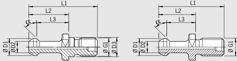
Version with ground pilot is used to help consistently locate the pull stud in the tool holder. Great for runout accuracy, balance repeatability and machine tool draw bar consistency.
