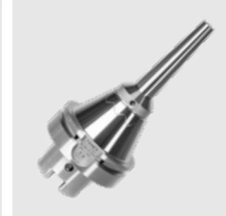
**Power Mini Shrink Chuck is perfect for 5-axis machining of parts that are difficult to access. Very slim at the top like the HAIMER Mini Shrink Chucks, the Power Mini Shrink is reinforced at the base. This allows for efficient milling with an angled tool, even at long protruding lengths.**
