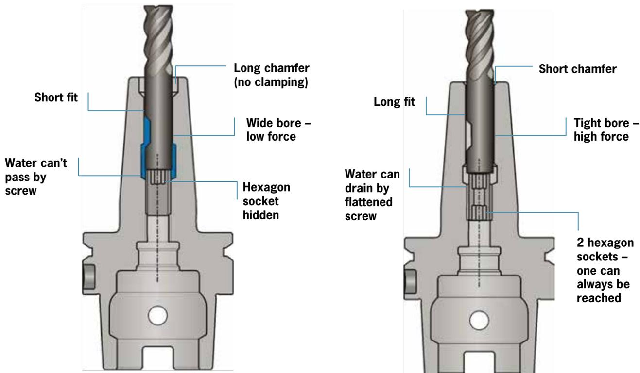
Comparison Shrink Fit Clamping Torque
